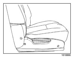
Lift the recliner lever, located on the outboard side of the seat, up fully and fold the seatback forward until it disengages.
